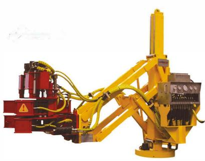
LM-120 Iron Roughneck is widely used during land and marine petroleum drilling operation, LM-120 Iron Roughneck is a wellhead instrument for operating makeup and breakout on drilling string (drill pipe, collar, casing and various tool joints) with caliber size of 3 1/2" ~9 5/8". It can greatly reduce labor intension of workers while operating trip out and trip in on drilling platform, and also improve the operation safety and efficiency.
